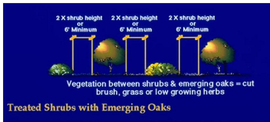
Figure 4. Shrub island spacing. Design groups of plants small enough to provide horizontal separation between groups. This allows proper maintenance and helps slow the spread of fire. Each shrub or group of plants should measure no wider than two times its height, or less than 120 square feet (or 6 feet x 20 feet). The space between groups should be greater than three times the height of the shrubs.
