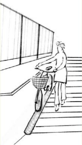
Maximum protrusion from wall for bicycle ramp: 4 inches
